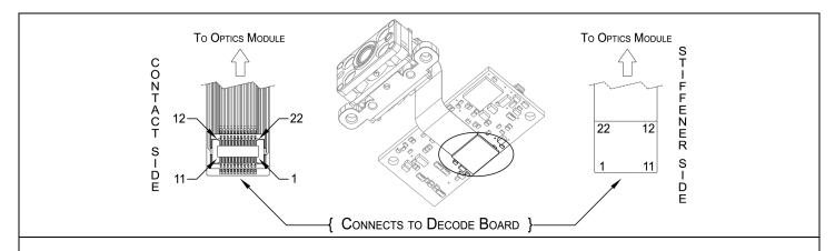
Figure 37. Flex Cable Pinout (Decode Connector End)
